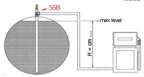
to open the valve at certain valvue of the pressure that, to make it easy, is marked with grooves on the spindle. These grooves are related to the exact height H of the diagram S that shows the tank and the dispenser.
